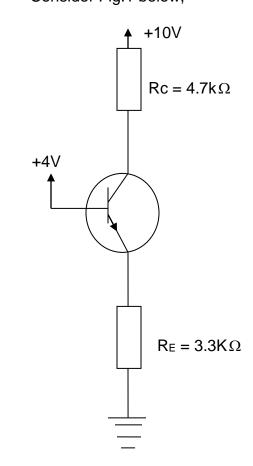
Given that  $\beta = 100$  and  $V_{BE} = 0.7V$ , calculate;
